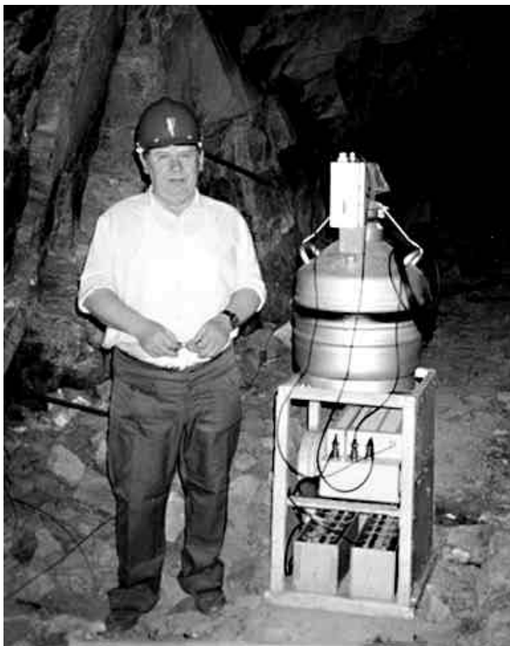
Figure 22. Radioactive gas sampling equipment used at a tunnel in Degelen mountain by the Russian Institute for Radiation Safety. The person in the photograph is Dr. Yuri Dubasov of the Khlopin Radium Institute, St. Petersburg.
